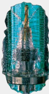
The „Cool down“ machines are a combination of induction shrinking technique and liquid cooling. Due to the all-in-one solution both the shrinking and the cooling process are effected in one position. This type of cooling makes a tool change in record time possible.
