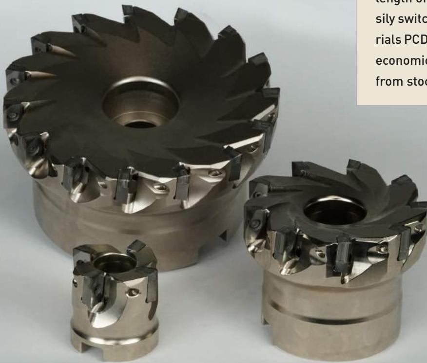
Our face and shoulder cutters have been specially designed for economical use with diamond and CBN inserts. You have the possibility to realize a high chip removal. Furthermore you can be very flexible due to the indexable insert solution, with a cutting edge length of 3mm and 7mm. You can easily switch between the cutting materials PCD, CVD-D and CBN. This highly economical solution is available from stock from ø32,00 - 100,00 mm.
